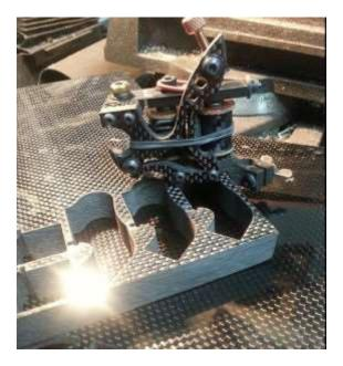
Carbon fiber is a material that may be easily machined with a CNC machine– photo shows a tattoo machine made from carbon fiber.
