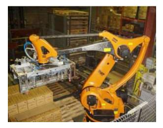
KUKA automated machine arm made from carbon fiber enables increased operating speed and reduces its weight at the same time, which results in reduced loading on bearings and other components subjected to wear.
