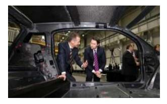
The carbon fiber car body enabled BMW to reduce the weight of IS model by 300 kg.
