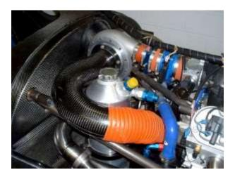
Carbon fiber is a perfect insulator- the above photo shows a carbon fiber turbine inlet.
