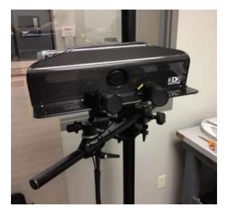
As, in practice, carbon fiber shows nearly zero heat expansion it is widely used in devices including 3D scanners.
